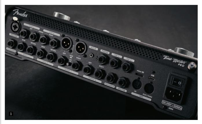
1. The Tone Master Pro's rear panel offers practically every connection you're ever likely to need. Highlights include no less than four assignable effects loops and two pairs of stereo outputs, with jack and XLR options 2. In a nod to the company's unrivalled heritage, Fender's Tone Master Pro features a miniature version of the iconic jewelled power indicator light, used on most of its valve amps for around seven decades
